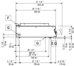
EQ = Equipotential screwG = Gas connection
